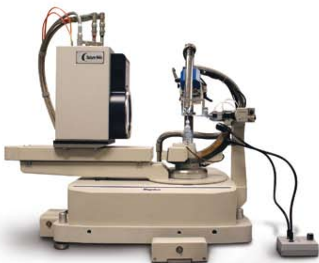
Saturn 944+ CCD detector Active area: 94 mm x 94 mm
