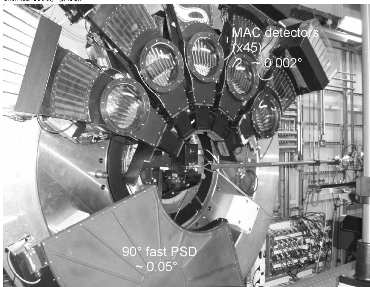
A close-up view of the powder-diffractometer on beamline I11. The high-resolution (MAC) detectors are mounted to the upper section of the diffractometer on the 2\theta axis while the position sensitive detector, shown in the lower region of the photograph, is mounted on the \delta axis which can be driven independently of 2\theta .
