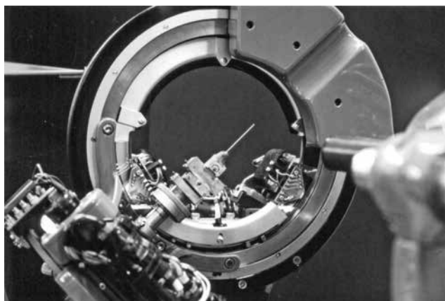
Fig 4. Close-up of the crystal on a Y290 showing the distinctive chi-circle of the Eulerian cradle.
