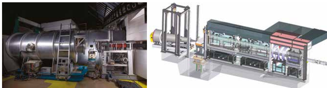
Figure 3. The reflectometers D17 (left) and FIGARO (right, layout of components) at the ILL ( http://www.ill.eu ).
