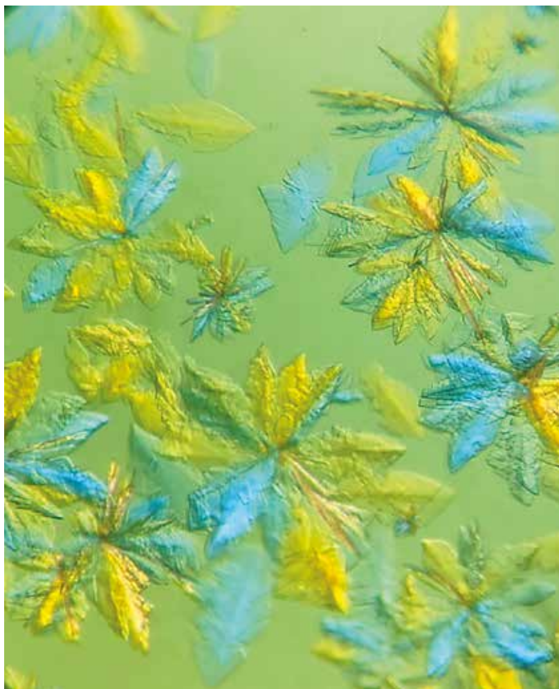
Figure 4. Microscopic view of the SARS-CoV-2 protease crystals grown in Oak Ridge National Laboratory's Protein Crystallization and Characterization laboratory (US). Once crystals reach a certain size and shape, they will be used in neutron scattering experiments.
