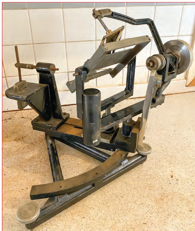
A historic X-ray precession camera. Thankfully the majority of workers who used these devices would have had the good fortune of using a more modern instrument. This photograph was very kindly provided by John Lisgarten (London).
