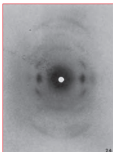
Diffraction patterns of unstretched silk (left) and stretched human hair (right). The similarity allowed deduction of the fact that both fibroin (in silk) and \beta -keratin (in stretched hair) have similar structures of extended chains of polypeptides. \alpha -keratin (in unstretched hair) has a shorter, folded structure, seen in the diagram alongside its \beta -form. Reproduced from Astbury and Woods, Philos. Trans. R. Soc., A , 232, 333 (1934).
