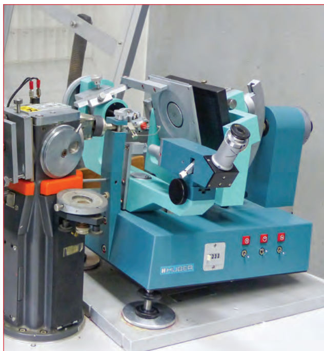
The editor's firm favourite was the Huber precession camera, mainly due to its simplicity and reliability. Note the annular metal screen in front of the black film cassette which, if set correctly, ensures that only one layer of the reciprocal lattice is recorded. This photograph was very kindly provided by Wolfgang Donner (Darmstadt). The instrument shown has a silver X-ray tube ( \lambda = 0.56 \text{ \AA} ) and a graphite monochromator, the film of old being replaced by a modern image plate. This precession camera is used both for educational purposes and for overview scans of diffuse scattering.
