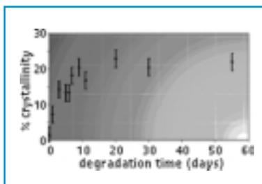
Figure 2: Changes in polyglycolide crystallinity during polymer degradation, calculated from the WAXS profiles.
