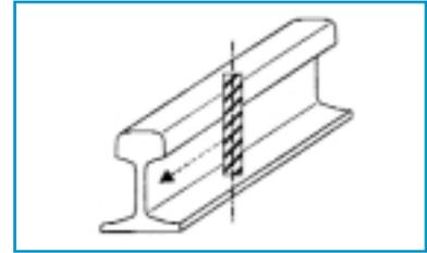
Figure 1. The rail and the plane along which the measurements have been performed. The arrow shows the direction of the longitudinal strain component.
