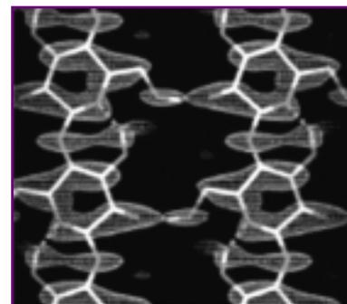
Figure 2. 2Fo-Fc map calculated from cellulose II. The neutron fibre diffraction data were recorded on instrument D19 at the Institut Laue Langevin, Grenoble (see Langan, Nishiyama, Chanzy, *J. Am. Chem. Soc.* 121(43), 9940)
