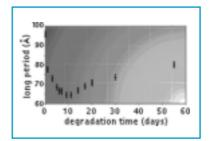
Figure 1: The long period of polyglycolide calculated by Bragg analysis of the Lorentz-corrected SAXS peak.
